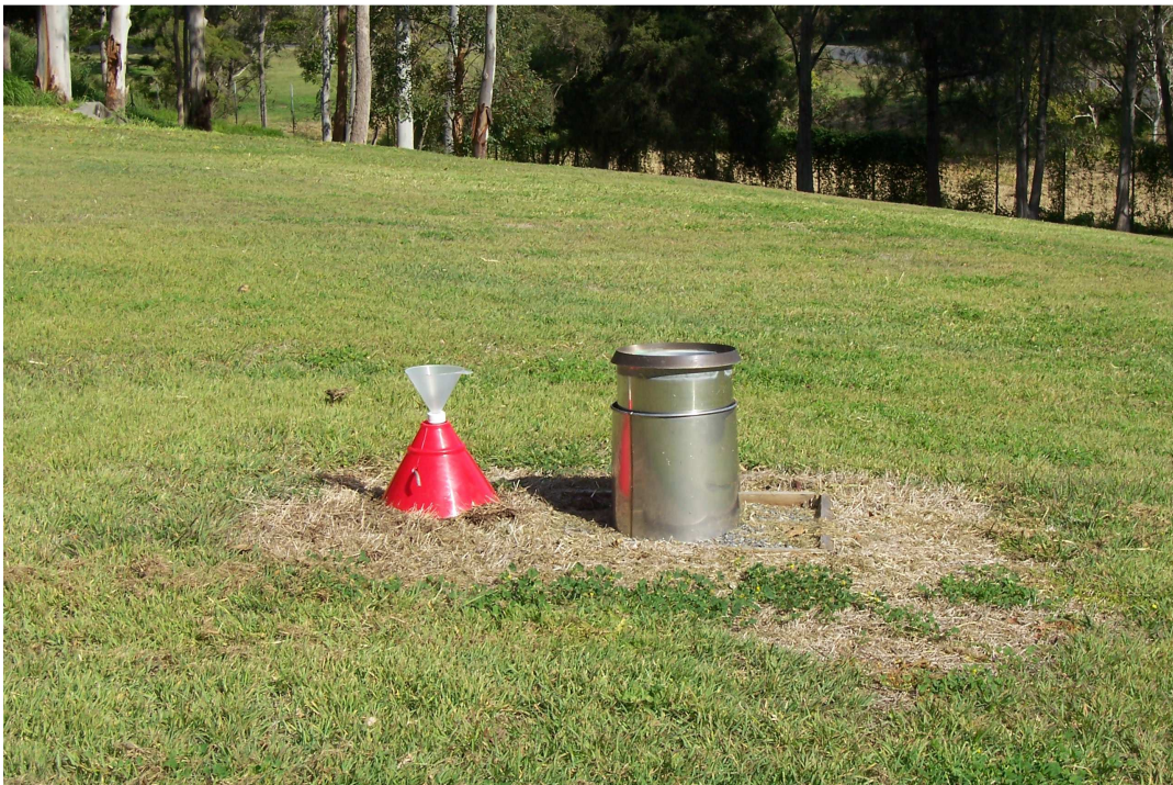
Figure 3. Rainfall collector (left) deployed in the field sitting next to a rain gauge (right)
